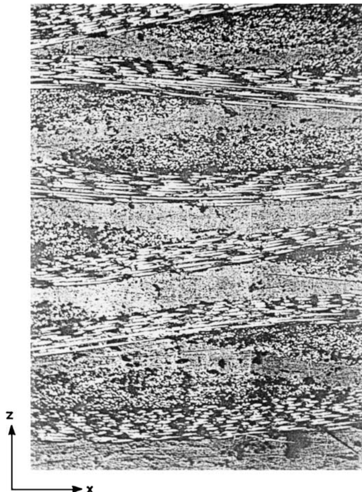
Figure 2 Photomicrograph of a typical plain weave fabric laminate cross-section.
